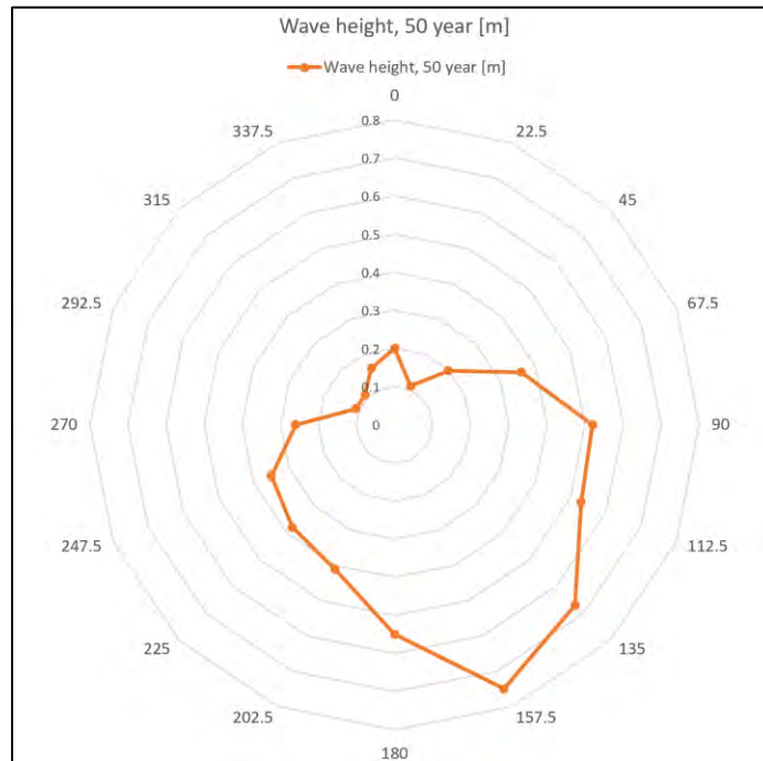
Figure 16 Maximum wave height at 50- year return period and direction [from]- Whycocomagh Bay - Marine Finfish Lease – 0600
